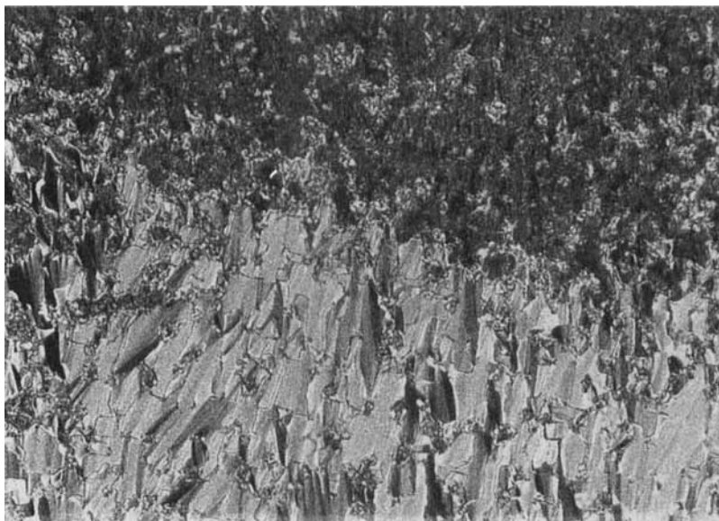
Figure 3. 14-13NCu. Smectic C phase, fan and schlieren textures. T = 390 K. Crossed polarizers.
